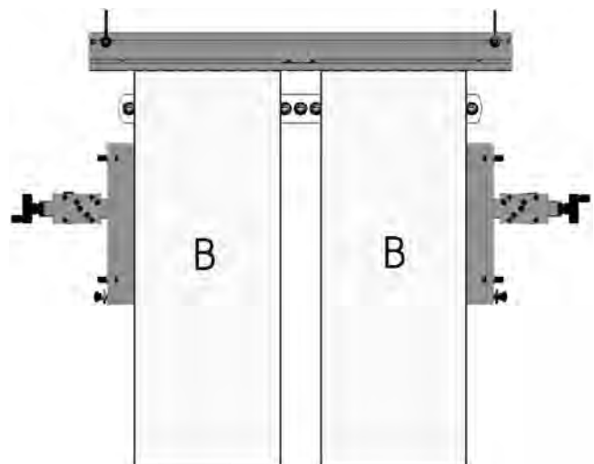
Simultaneous drilling of two side panels (drilling head at 90°)
